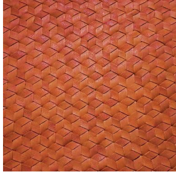
Figure 8. Triaxial weave structure of leather.
