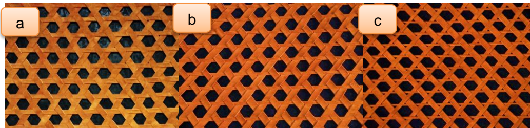
Figure 11. leather triaxial weave structure with space between axes (a) axes width 12mm, (b) axes width 12mm, 8 mm, (c) axes width 4mm, 8mm, and 12 mm.
