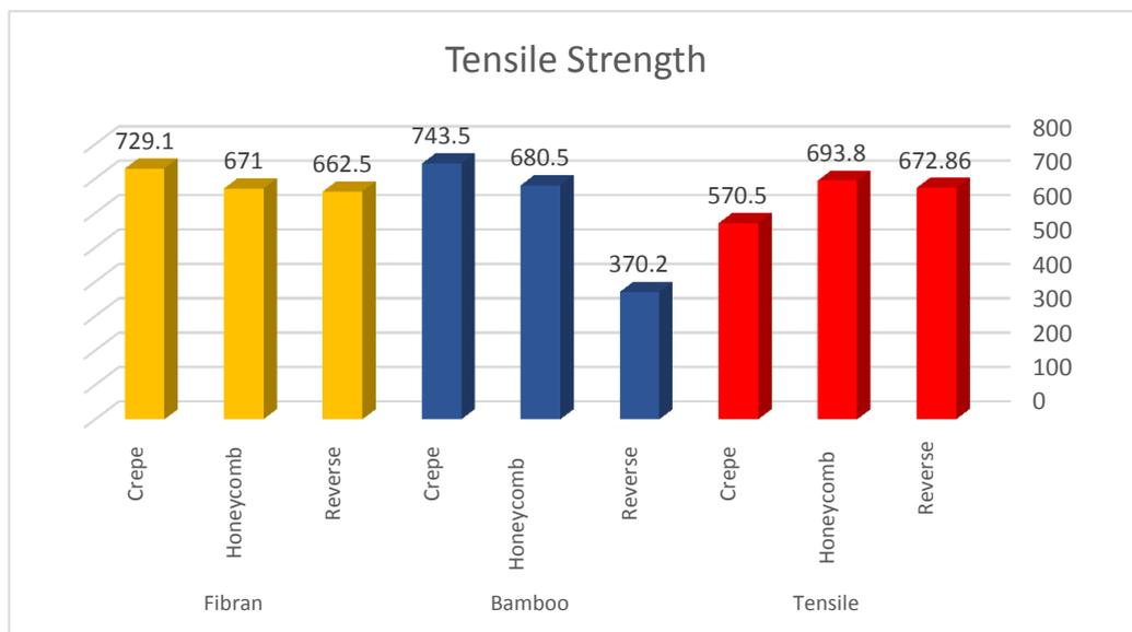
Figure (2): Averages of the raw materials treated with silver nanoparticles for the weaving constructions in the tensile strength test (Newton).
