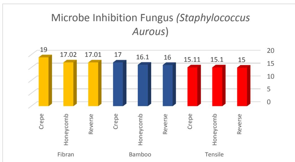
Figure (6): Averages of the raw materials treated with silver nanoparticles for the weaving constructions in the test of microbe inhibition fungus (*Staphylococcus Aureus*)
