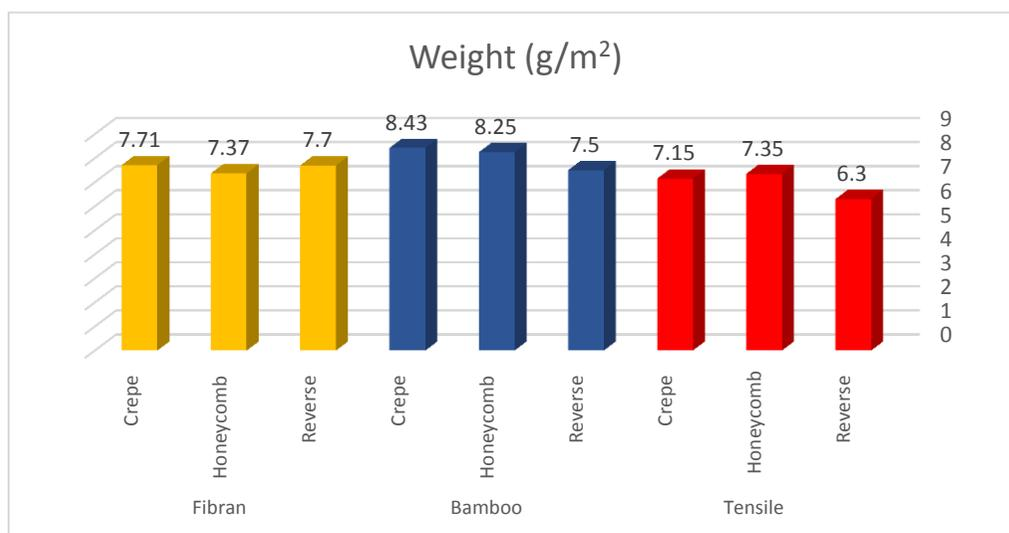
Figure (4): Averages of the raw materials treated with silver nanoparticles weaving constructions in the weight test (g/m<sup>2</sup>)
