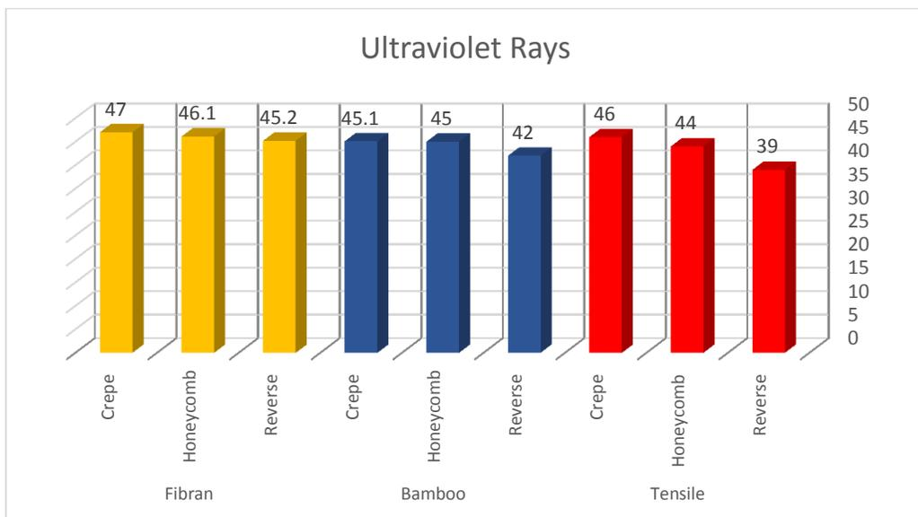
Figure (1): Averages of the raw materials treated with silver nanoparticles for the weaving constructions in the (UPF) test.
