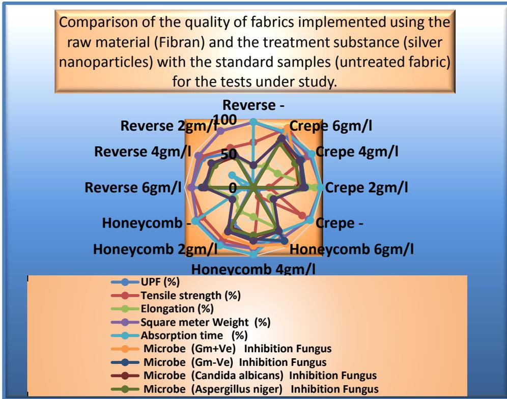
Figure (12): Comparison of the quality of fabrics implemented using the raw material (Febran ) and the treatment substance (silver nanoparticles) with the standard samples (untreated fabric) for the tests under study.
