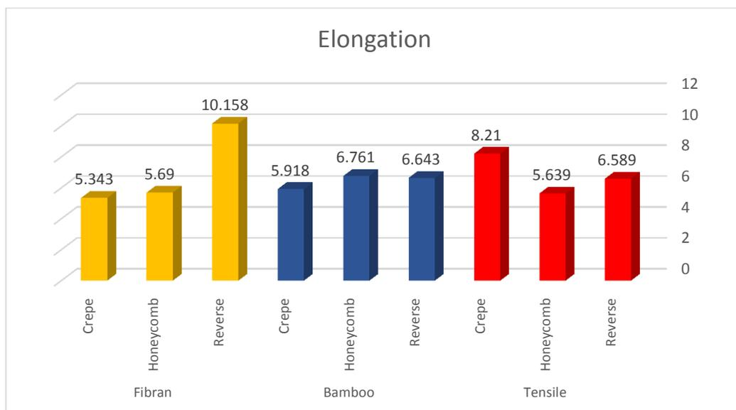
Figure (3): Averages of the raw materials treated with silver nanoparticles for the weaving construction in the elongation test (%).
