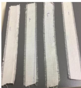
Figure (2): under study frayed samples of fabrics
