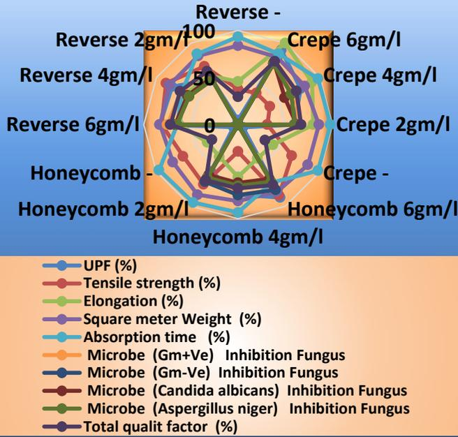
Figure (11): Comparison of the quality of fabrics implemented using raw material (Bamboo) and treatment substance (silver nanoparticles) with standard samples (untreated fabric) for the tests under study.
