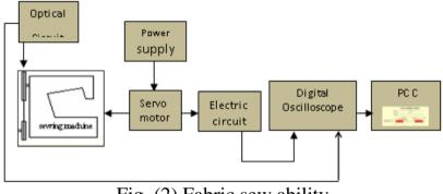
Fig. (2) Fabric sew ability Sew Ability Tester (ST2), [3-5].
