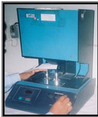
Image5) shows the measure of the tensile strength of the paper.
