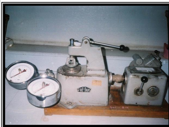
Image7) Device to measure rupture resistance.
